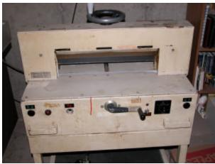
This ancient looking machine is an electric paper cutter. Once the books are assembled, they need to be cut in half, and the halves put together to form a complete book. Then, all 1,000 copies will be trimmed on the remaining three sides for evenness. In total, about 300 cycles of this blade will be required for all of the books to be ready for binding.
