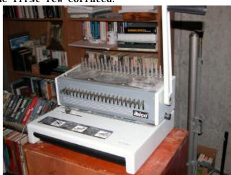
This is a manual punch-and-bind machine. Once the books are cut and trimmed, they all have to be punched (2-3 punches per book) to make holes for the binding rings. When finished, between 2,000-3,000 punch strokes have been made.
